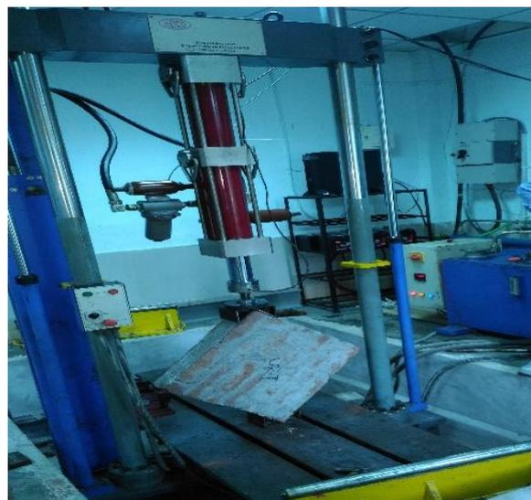
**Fig.3.** Servo Hydraulic Dynamic-Static Actuator
